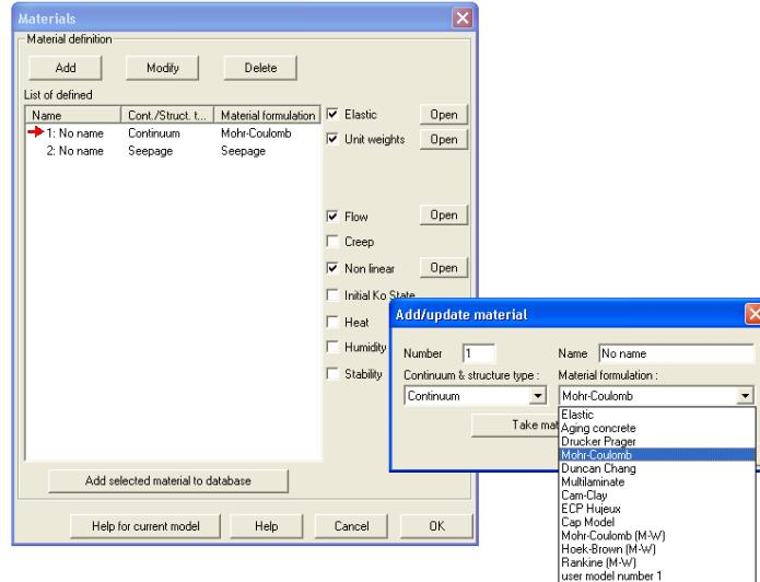
Set the Elastic, Unit weights, Flow and Non-linear properties by clicking ‘Open’ according to the values in Table 1. Note that since no material has been specified during the construction of the mesh, the material n.1 is applied by default to all elements.
