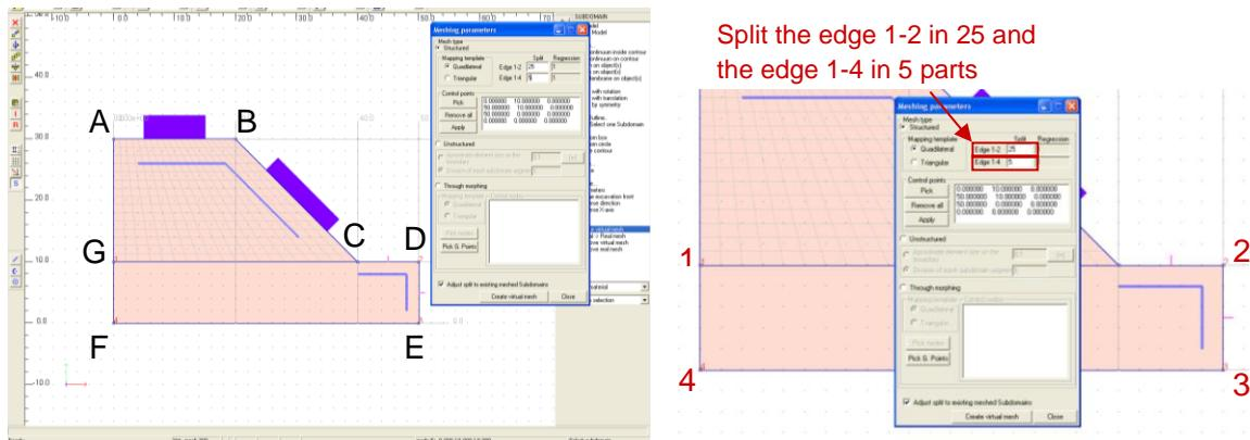
The created virtual mesh has to be converted in a real mesh selecting on the right menu ‘MACRO MODEL > Subdomain > Mesh > Virtual → Real mesh’ and clicking inside the two subdomains. Note that the hydraulic boundary conditions specified in the macro model are correctly applied to each element of the real mesh.
