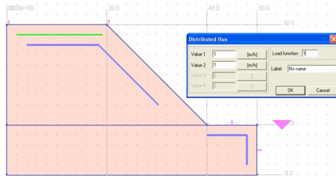
Repeat the same procedure for the edge BC assigning 0.71 to Value 1 and Value 2, and 1 to the load function.
