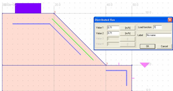
Not assigning any hydraulic boundary condition to the edges AF and FE is equivalent to identify them as impermeable boundaries.
