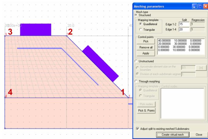
Click inside the lower subdomain. In this case the control points are not automatically identified since the subdomain contour has more than 4 points (5 in this case). The control points have to be identified using the ‘Pick’ command in the ‘Meshing Parameters’ window and clicking on the four subdomain corners (GDEF). Split the edge GD (1-2 in the figure) in 25 parts and the edge GF (1-4 in the figure) in 5 parts. Click on ‘Create virtual mesh’.
