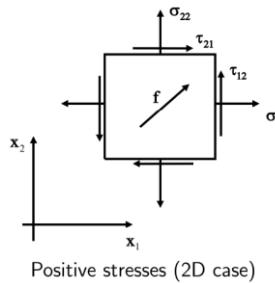
Sign convention for the fluid pressures is adopted consistently with stress field convention, i.e. positive pressures ( $p > 0$ ) are for tension, negative pressures ( $p < 0$ ) are for compression. Same convention applies for the effective stress (positive in tension). Sign convention for the strains is adopted consistently with stress field convention, i.e. tensile strains are positive.
