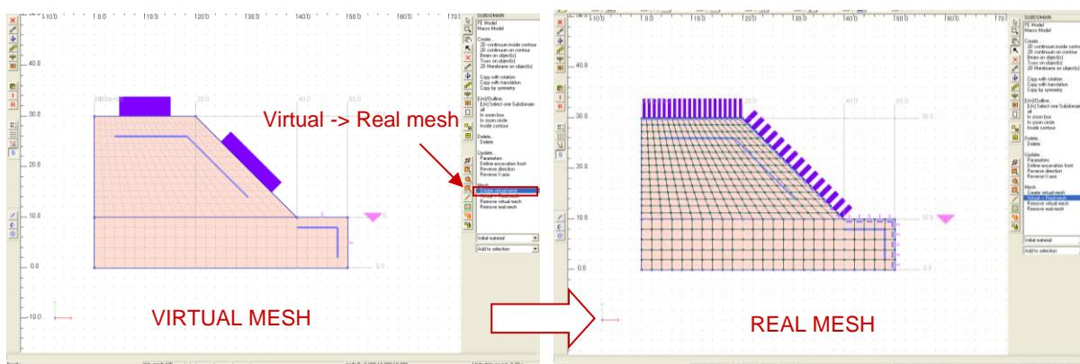
Once the mesh has been created, kinematic boundary conditions have to be applied. The preprocessor offers a simple way to apply classical displacement boundary conditions that prevent horizontal displacements for the nodes on the lateral edges of the domain, and any displacements for the nodes of the domain bottom. To do this, select on the right menu ‘FE model > Boundary conditions > Solid BC > On box’.
