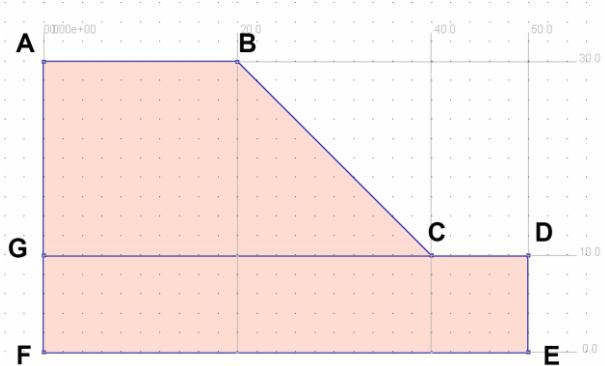
A fixed piezometric head equal to 10 m will be assigned to the edges CD and DE, equivalent to a hydrostatic condition with the water table coinciding with the river level. Highlight both edges by means of the 'Select edge in zoom box' icon and use on the right menu the command 'MACRO MODEL > Pressure BC > Fluid head on the selected edges'. Input 10 (m) in the 'Fluid head' cell and press OK.
